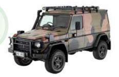
The role of these variants is to provide high-mobility general purpose load transport. These variants are an essential component of support, sustainment, deployment and redeployment structure and are used to transport combat supplies, materiel and replacement combat systems. These vehicles will accommodate two people; a driver and a co-driver.
