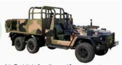
The role of the Truck, Light, Surveillance and Reconnaissance is to provide high-mobility transport to Regional Force Surveillance Units for conducting wide area surveillance tasks. The vehicle, when on patrol, will normally be operated by three personnel, comprising of a driver, co-driver and rear observer.
