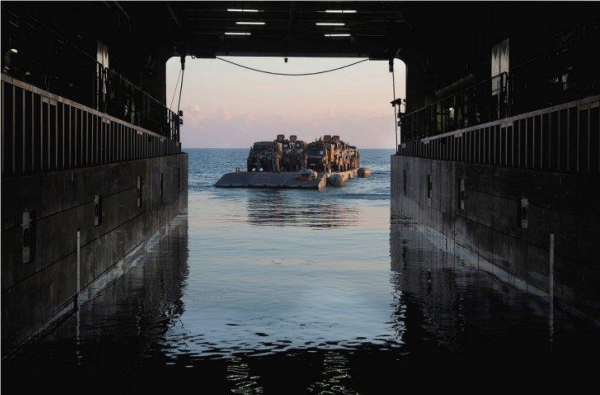
LHD HMAS Choules's Mexe-Float, loaded with Australian Army vehicles, sails from the stern door ramp of the ship's vehicle deck during Exercise 'Talisman Sabre 2015'. ( Australian DoD)
