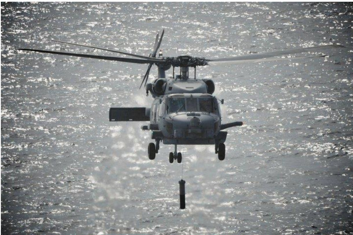
A Royal Australian Navy MH-60R maritime helicopter conducts functional testing of its newly fitted AN/AQS-22 Airborne Low Frequency Sonar System off the coast of Jacksonville, Florida, on 13 May 2014. As well as supporting the detection, tracking, localisation, and classification of submarine threats, the AQS-22 also performs acoustic intercept, underwater communications, and environmental data acquisition. (Australian DoD)
